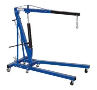
Capacity Dimensions Fold dimensions Min/max boom extension Hook heights with raised arm Hook heights with lowered arm Front opening Net weight 1000 kg 1800 x 1000 x 1500h mm 800 x 860 x 1600h mm 680 ÷ 1220 mm 2100 mm (a 1000 kg | 2550 mm (a 250 kg 0 mm (a 250 kg | 480 mm (a 1000 kg 800 mm 90 kg
