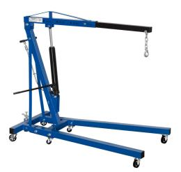
Capacity Overall sizes Fold dimensions Min/max reach Hook heights with raised arm Hook heights with lowered arm Front opening Net weight Packaging dimensions Gross weight EAN Code 1000 kg 1800 x 1000 x 1500h mm 800 x 860 x 1600h mm 680 - 1220 mm 2100 mm @ 1000 kg | 2550 mm @ 250 kg 0 mm @ 250 kg | 480 mm @ 1000 kg 800 mm g 90 kg 1550x410x220 h mm 95,00 kg 8012667184193
